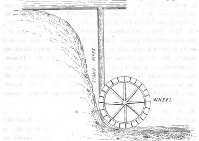
With wheels constructed on this principle a very great amount of power is obtainable when there is only a small supply of water, and the high velocity which they acquire renders them peculiarly well adapted for driving rolling mills. This kind of wheel differs from the turbine, and suggested itself to me during the progress of the works.
