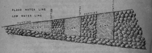
23. A series of dry rubble walls have been built in an oblique direction across the river, with a slight curve upwards, according to the following Plan, and as shown in the Section above. At the upper sides of these walls tatties made of grass and bamboos were fixed and the spaces between the walls were then filled in with clay and mud and soil—the whole was then covered with other tatties, and a covering of soil and
